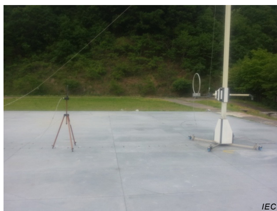
a) Measurement at coaxial direction at 3 m
